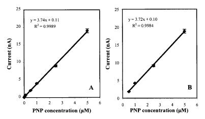
Fig. 4. Calibration plot for PNP amperometric microbial biosensor. A) in 50 mM pH 7.5 citrate-phosphate buffer and B) in Lake Elsinore water filtered and adjusted to pH 7.5, at room temperature with 0.03 mg cell loading, applying +0.4 V to working electrode vs. the Ag/AgCl reference. Data are given as mean  $\pm 1$  SD for three experiments.
