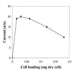
Fig. 2. Effect of cell loading on biosensor response to 5  $\mu$ M PNP in 50 mM pH 7.5 citrate-phosphate buffer at room temperature. Operating potential: +0.4 V (vs. Ag/AgCl). Data are given as mean  $\pm$  1 SD for three experiments.
