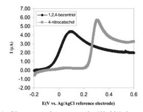
Fig. 1. Linear scan voltammograms for  $100 \mu M$  4-nitrocatechol and  $100 \mu M$  1,2,4-benzenetriol with carbon paste electrode in 50 mM pH 7.5 citrate-phosphate buffer at room temperature. Scan rate is 20 mV/s.
