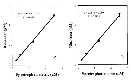
Fig. 5. Accuracy of amperometric microbial biosensor. A) in 50 mM pH 7.5 citrate-phosphate buffer and B) in Lake Elsinore water filtered and adjusted to pH 7.5, at room temperature with 0.03 mg cell loading, applying +0.4 V to working electrode vs. the Ag/AgCl reference. Data are given as mean  $\pm 1$  SD for three experiments.
