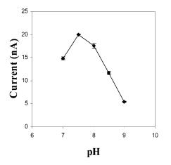
Fig. 3. Effect of pH (50 mM citrate-phosphate) on biosensor response to  $5 \,\mu M$  PNP with 0.03 mg cell loading at room temperature. Operating potential:  $+0.4 \,V$  (vs. Ag/AgCl). Data are given as mean  $\pm 1$  SD for three experiments.
